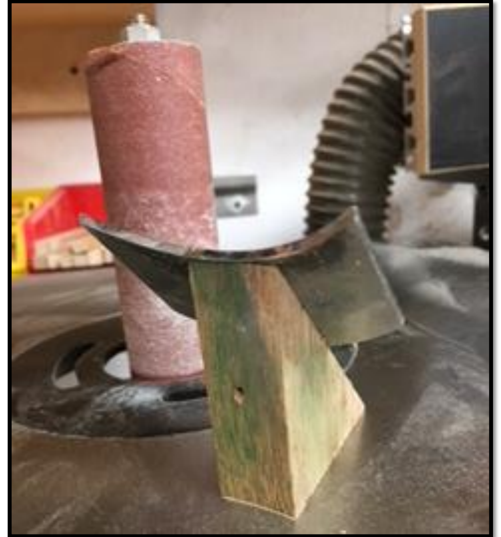
Step 4. Grind the angle until the whole surface has been ground.
