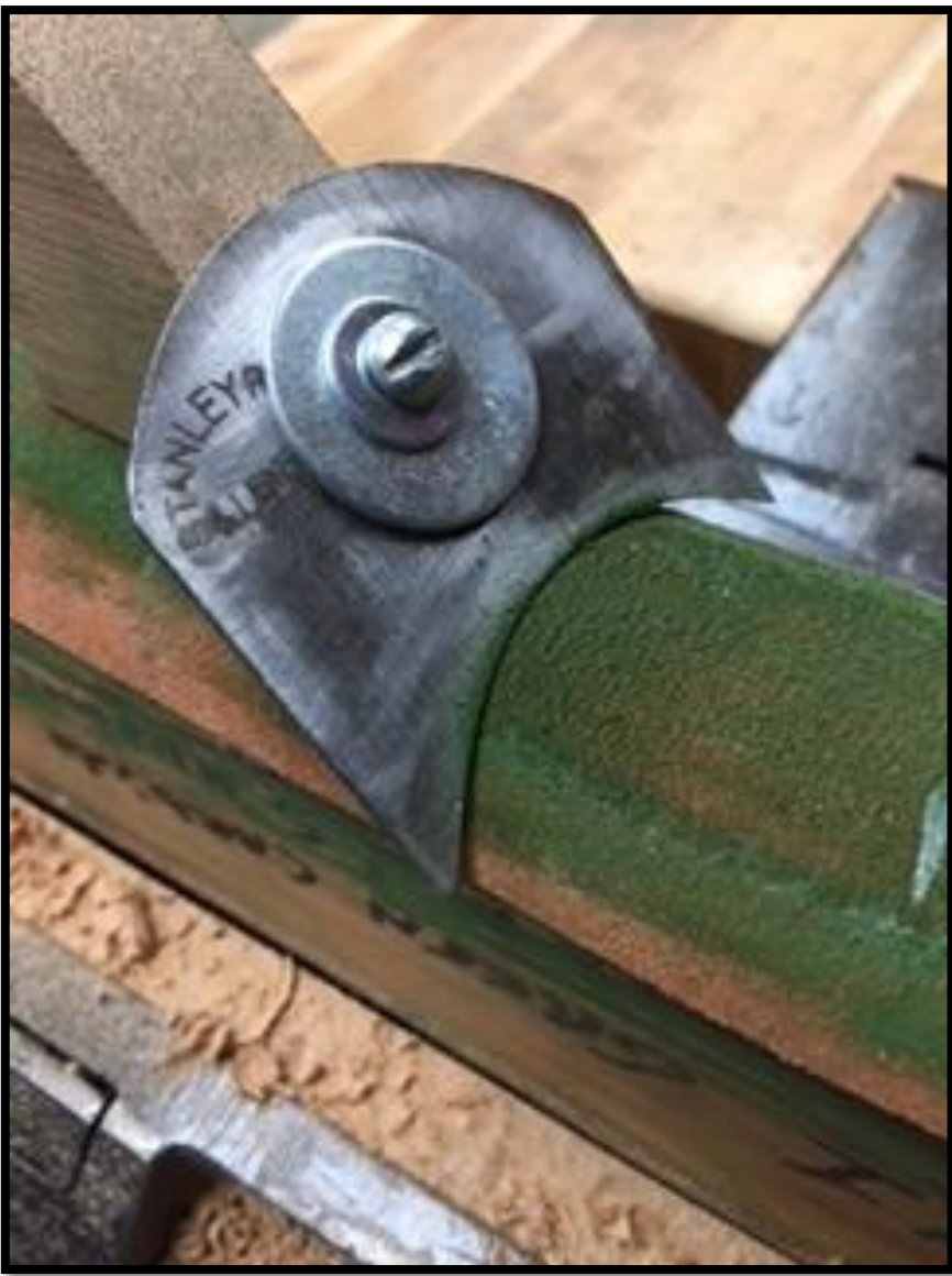
Step 7. Hone cutting edge until the entire surface is smooth to a mirror finish.
