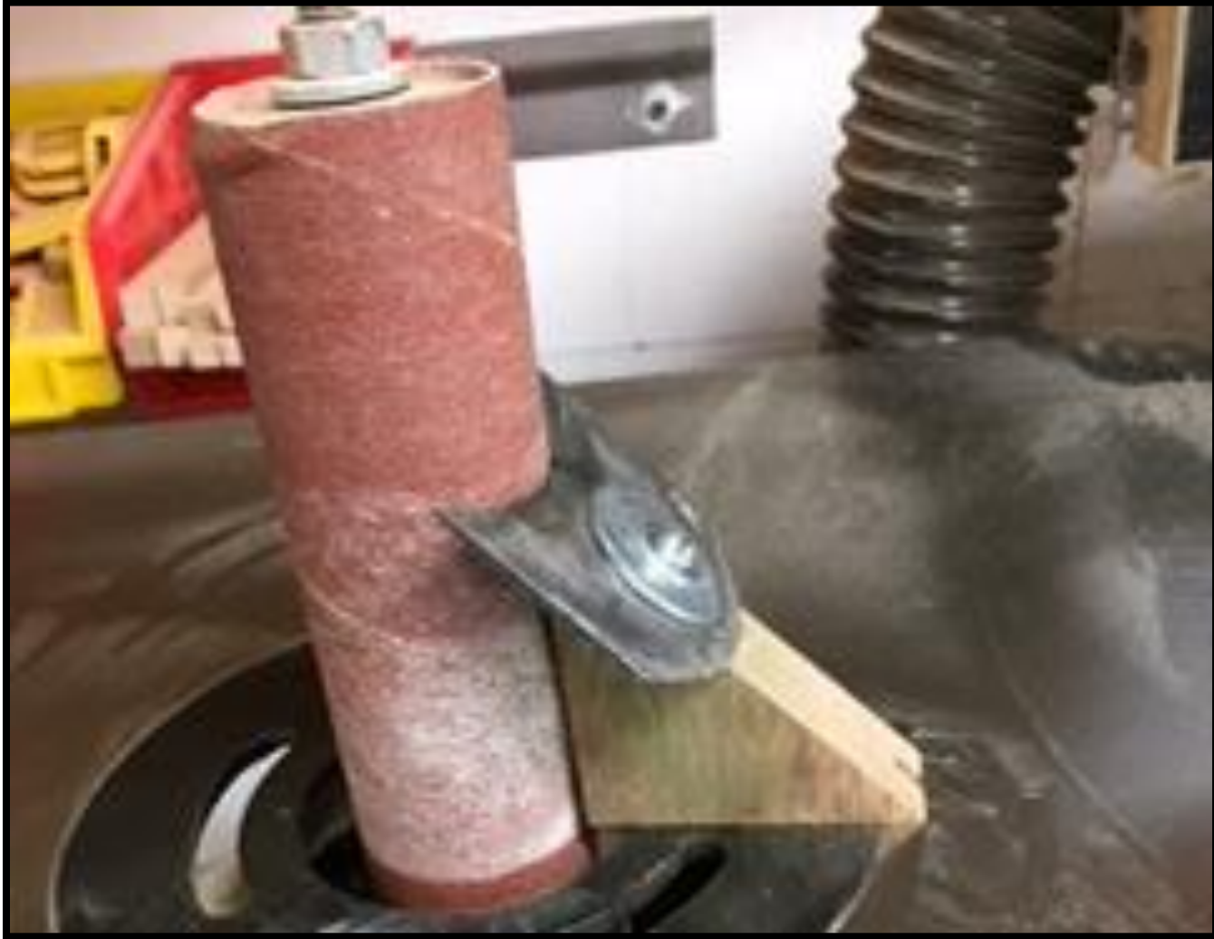
Step 3. Attach the iron to the jig and then install large drum spindle to your spindle sander or use a drill press.
