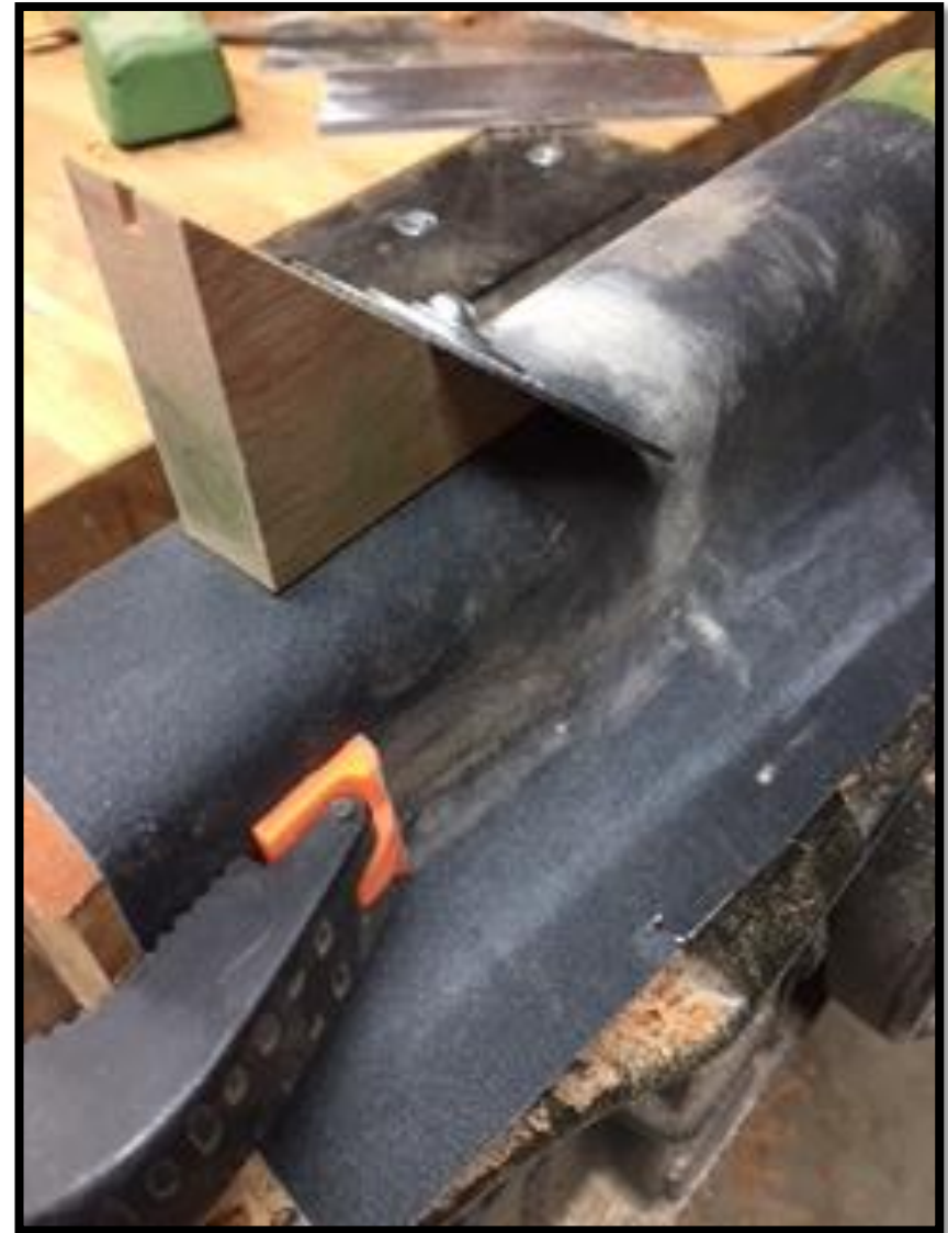
Step 6. Sand the edge 220-600 grit pulling backward on the abrasive paper. Finer abrasive paper can be used.
