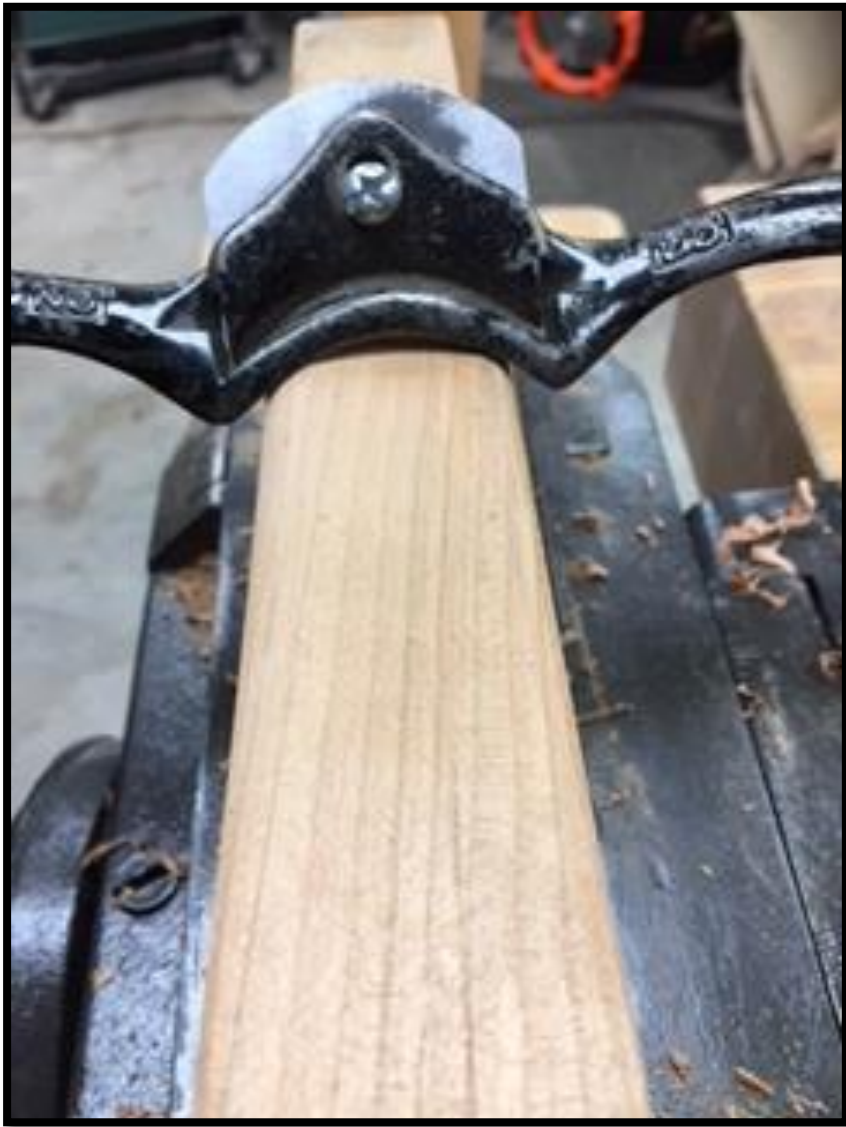
Step5. Profile the edge of a wide board and then glue on a piece of leather (Animal or epoxy glue) to it.
